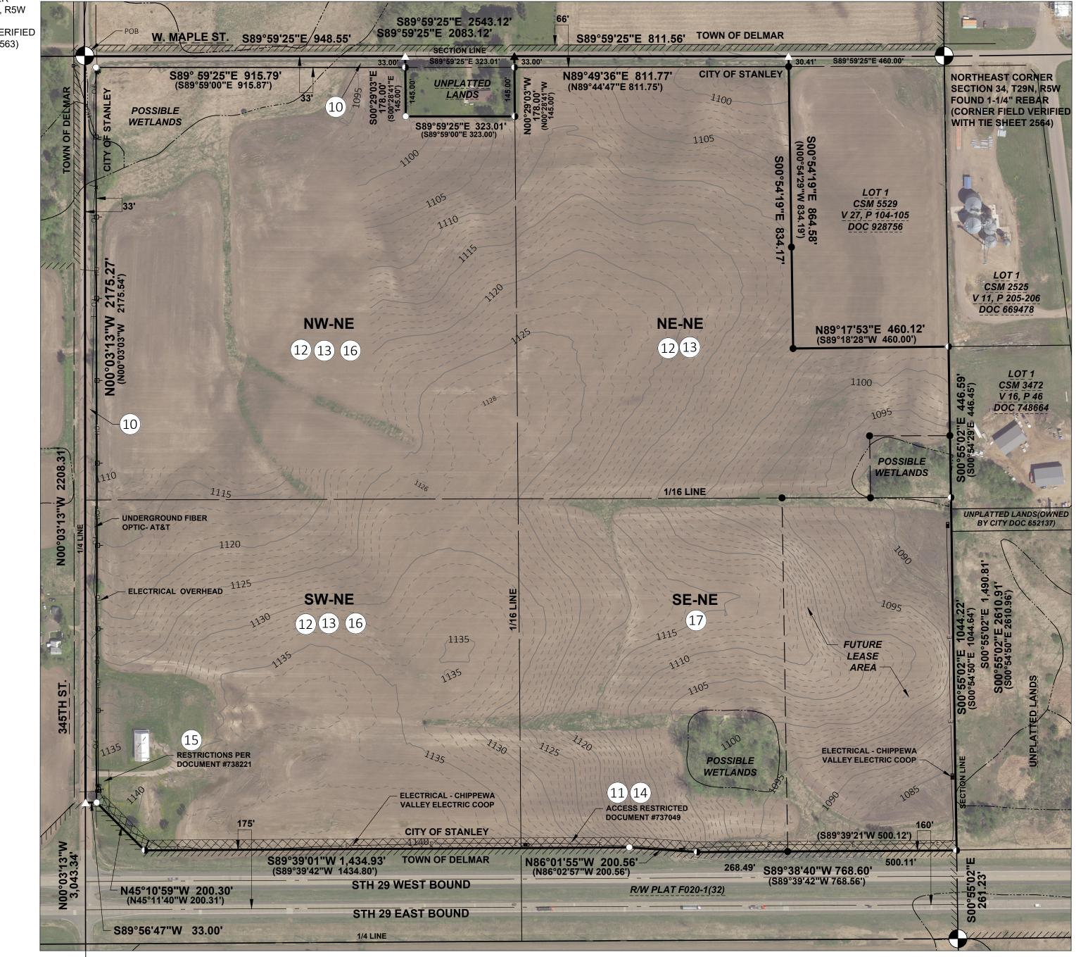
NORTH 1/4 CORNER SECTION 34, T29N, R5W FOUND MAG NAIL (CORNER FIELD VERIFIED WITH TIE SHEET 2563)
